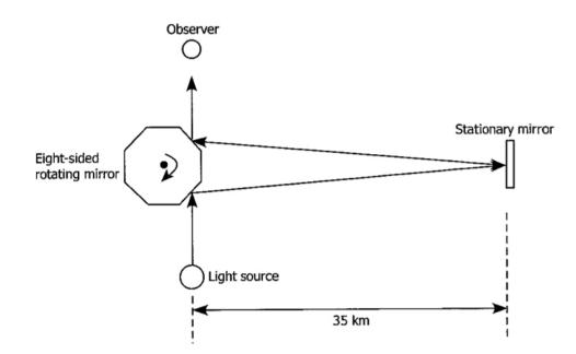
The distance between the mirrors was measured to be  $35\ 385.5\ m$ , accurate to about one part in seven million. This was a much larger distance than the  $10\ m$  or so that Foucault used. The rate at which the mirror was rotating was measured accurately using a stroboscopic comparison with an electric signal at standard frequency.
